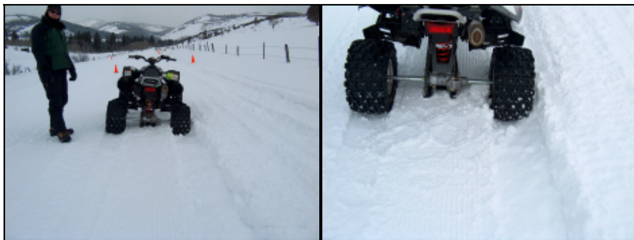
Photos 170 and 171: The vehicle got off the edge of the compacted base and got stuck
