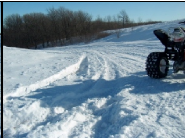
Photos 50 and 51: ATV flipped end-over-end when its right tires got off the compacted trail base
