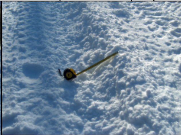
Photo 40: Berm created by fast pass-bys
