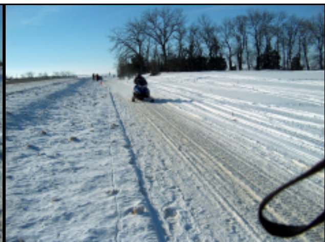
Photo 16: Surface chew from fast pass-by
