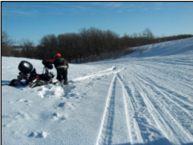
Photos 50 and 51: ATV flipped end-over-end when its right tires got off the compacted trail base
