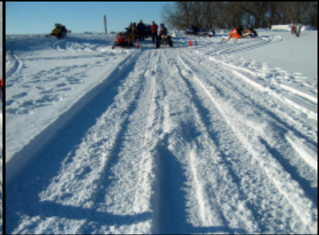
Photo 9: Tracks and snow piles from acceleration
