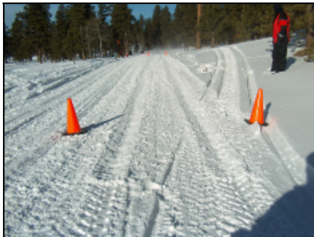
Photo 59: Tire impressions from an aggressive start
